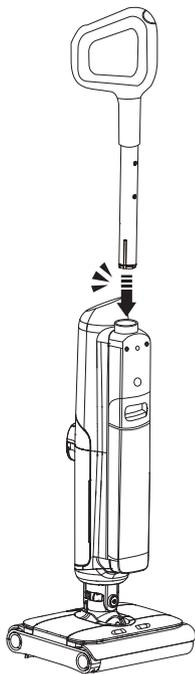
1.2 Disassembly: Use a pen-like hard object to press down the latch inside the hole on the back of the machine, and at the same time, pull up the main unit handle to remove it.
